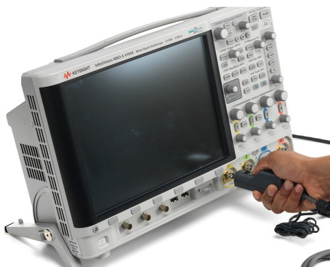
Figure 2 Connecting the Probe to the Oscilloscope
