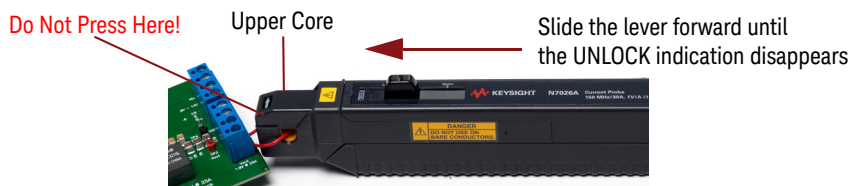
Figure 4 Use the Opening Lever
