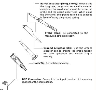
Ground Spring: Connect to the probe head for grounding and better high frequency response.
