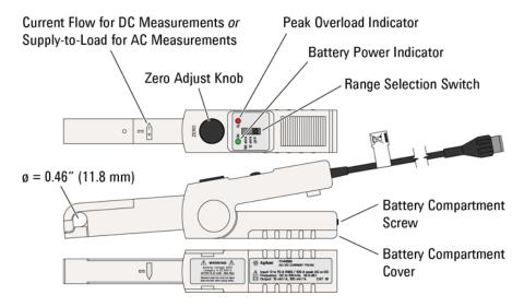
Figure 1 **Control and Connector Identification**
