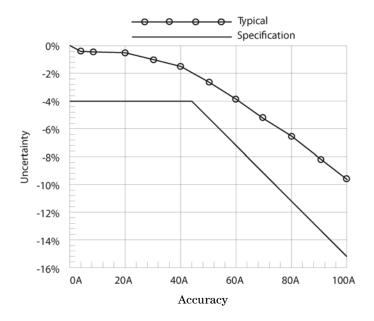
Figure 4 Linearity for a DC Signal Range 10 mV/A
