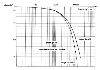
Figure 3 Typical Phase Shift Response Curve
