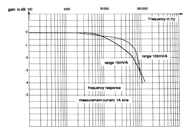
Figure 2 Typical Frequency Response Curve
